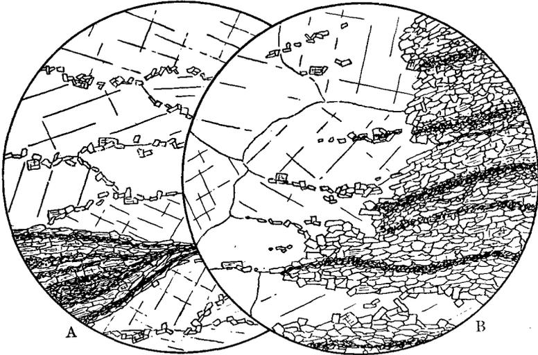
FIG. 4. A. Halite-anhydrite-rock with deformed lenticle of anhydrite-dolomite-rock. The halite grains are markedly flattened. Halite-anhydrite zone, 4142-44 feet.  $\times 14$ .
