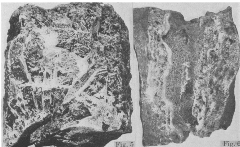
FIG. 5. Halite-anhydrite-rock with pseudomorphs after swallow-tail twins of gypsum. The surface of the core has been etched by the drilling water, the halite (dark) being partially dissolved. Halite-anhydrite zone, 4108-10 feet.  $\times \frac{1}{2}$ .
