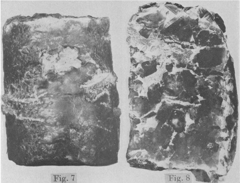
FIG. 7. Anhydritic layers faulted and contorted due to recrystallization of adjacent halite. Etched surface of core. Halite zone, 4094-96 feet.  $\times \frac{1}{2}$ .
