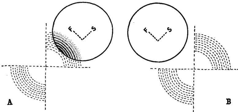
FIG. 2. Interference figure of calcite cleavage flake, using high-order plate.
