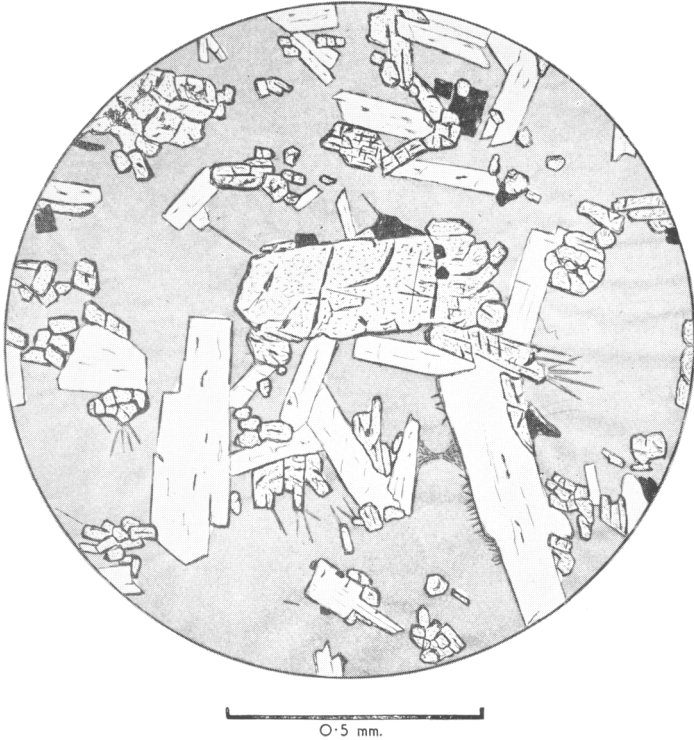
FIG. 1. Tholeiite composed of plagioclase, pyroxene, magnetite, and glass. The large crystal in the centre of the field is hypersthene rimmed by a clinopyroxene.
