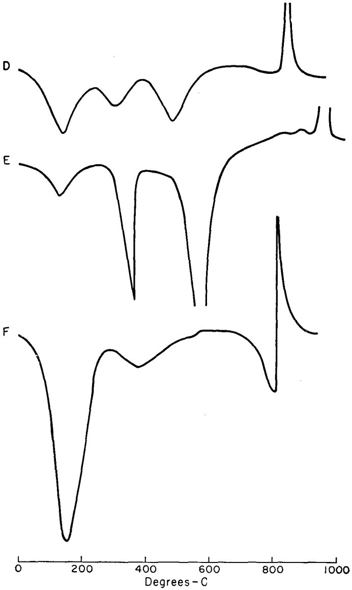
FIG. 6. Differential thermal analysis curves: D, Palygorskite, Attapulugus, Georgia; E, Halloysite (with gibbsite), Bedford, Indiana; F, Sepiolite, Vallecas, Spain.
