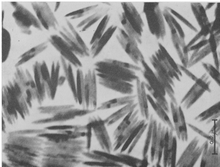
FIG. 5. Somatoid particles of \beta -FeOOH showing parallel association.
