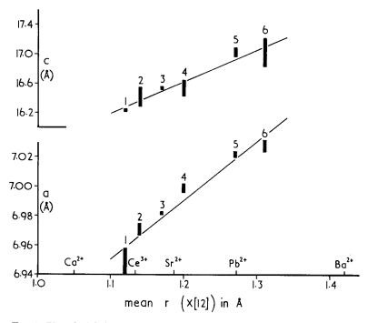
FIG. 4. Plot of triple hexagonal unit-cell dimensions in the goyazite series against mean radius of cations on twelve-fold coordinated sites. The numbering corresponds to that of the columns of table V. The size of the plotted points represents the error of the measurements. The radii of the principal X cations are indicated by their symbols.
