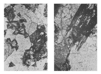
FIGS. 1 and 2: FIG. 1 (left). Strontian florencite rhombohedra in a matrix of ankerite and strontianite. Kangankunde Hill, Nyasaland. Plane polarized light,  $\times$  100. FIG. 2 (right). Fine-grained cerian goyazite (dark) intergrown with quartz and baryte in a dolomitic matrix. Wigu Hill, Tanganyika. Plane polarized light,  $\times$  20.
