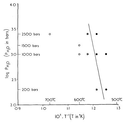
FIG. 3. Hydrothermal stability of strontian florencite. Open circles: decomposition product only. Shaded circles: partial decomposition. Solid circles: florencite persists.
