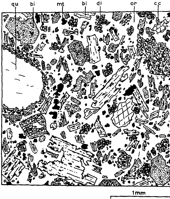
FIG. 1. Minette (analysed, table I). Biotite ( bi ) flakes and numerous cross-sections are set in an orthoclase base ( or , no ornament) with grains of diopside ( di ) and magnetite ( mt ). Also present are scattered patches of calcite ( cc ) and a quartzite xenolith ( qu ) fringed by tiny diopsides.
