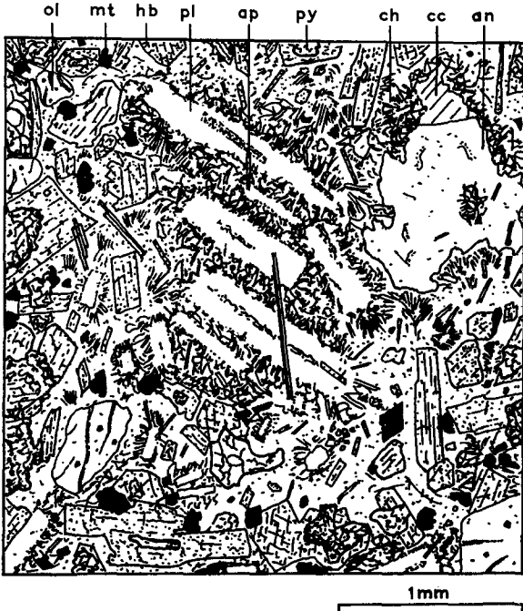
FIG. 2. Camptonite (analysed, table V, 2). At the centre of the ocellus, about 3 mm in diameter, analcime ( an ) is partly replaced by calcite ( cc ). Large laths of andesine-labradorite ( pl ) occur marginally in an altered, glassy base ( ch ) penetrated by apatite needles ( ap ). Prisms of brown hornblende ( hb ) fringe the ocellus and mantle titanite grains ( py ), which with bowlingite pseudomorphs after olivine ( ol ) are more numerous away from the ocellus.
