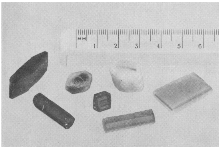
FIG. 5. Specimens of ruby and corundum crystals grown on seeds.
