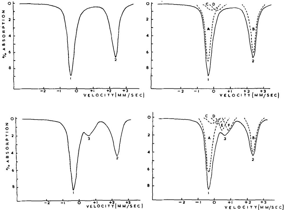
FIGS. 1 and 2: Fig. 1 (left). The Mössbauer spectra of: (a) (top), fresh biotite; (b) (bottom), weathered biotite. Fig. 2 (right). A pictorial representation of the interpretations given in table II for: (a) (top), fresh biotite; (b) (bottom), weathered biotite.
