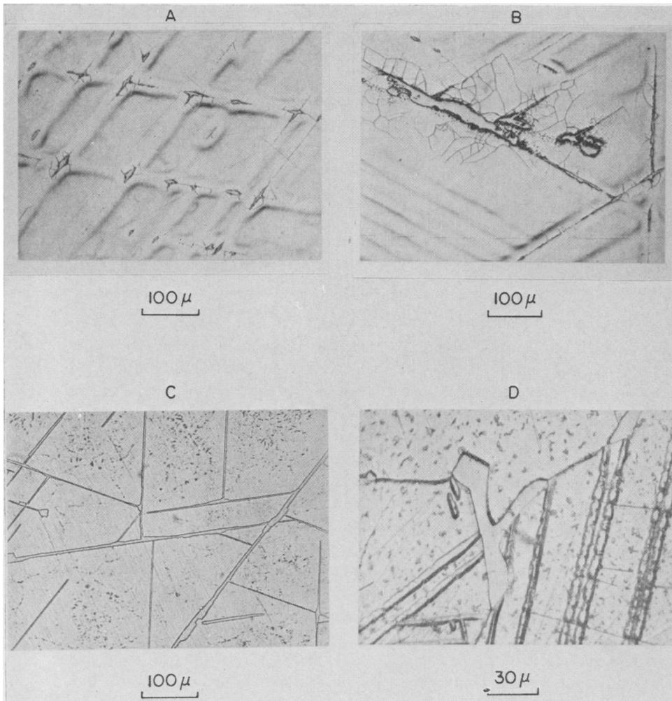
FIG. 1. A. Etched metal phase of Mount Egerton showing the 'pseudo-octahedral' structure and perryite inclusions. B. Perryite inclusions in the metal of Mount Egerton. C. Etched metal phase of Horse Creek showing lamellae of perryite inclusions. D. Etched metal phase of Norton County showing a Y-shaped perryite inclusion at the intersection of three kamacite crystals.
