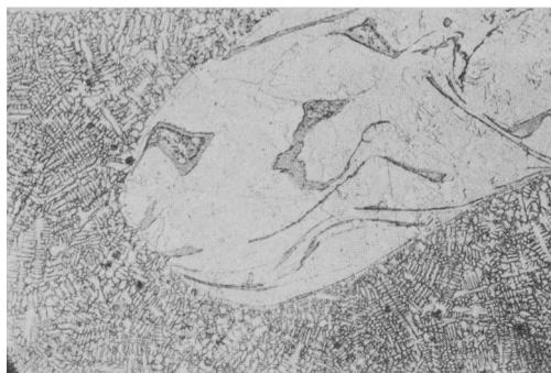
FIGS. 3 and 4: FIG. 3 (left). Map of the distribution of dendritic material,  $\alpha_2$  kamacite,  $\epsilon$ -kamacite, and troilite obtained by the microscopic examination of the section shown in fig. 1. FIG. 4 (right). Dendritic area in detail showing undissolved fragments of distorted and reheated metal. Field view  $0.17 \times 0.11$  mm. Nital etch.
