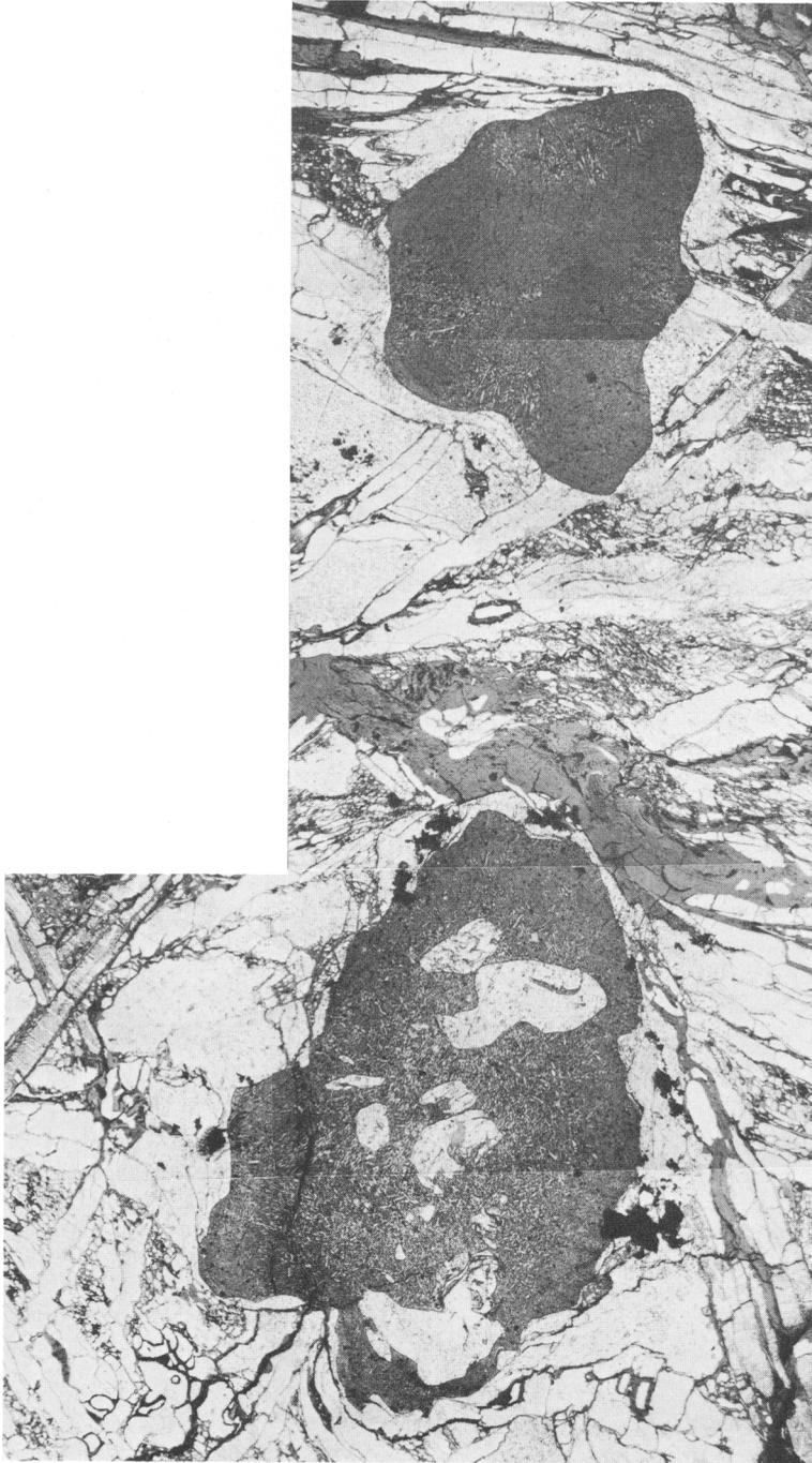
FIG. 2. Microstructure of the dendritic globules of fig. 1 and of the surrounding metal. Photo-mosaic, showing extensive corrosion, finest kamacite bands, and spheroidized plessite. Aureoles of reheated  $\alpha_2$  surround the dendritic globules but light etching does not clearly show the  $\varepsilon$ -kamacite. A corrosion filled crack runs through the larger globule. True length of this photo-mosaic field 3 mm. (See also fig. 3.)
