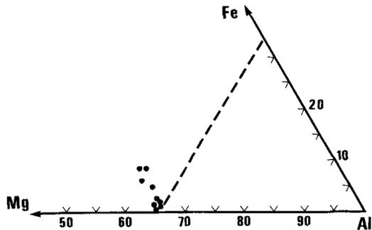
FIG. 1. A portion of ternary spinel plane expressed as atomic Mg-Al-Fe. The dashed line is the join  $MgAl_2O_4$  (spinel)- $FeAl_2O_4$  (hercynite). Shown by solid dots are the aluminian spinels found in the marbles.
