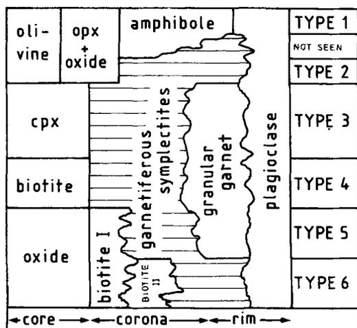
Fig. 2. Schematic representation of the six types of corona discussed in this paper.
