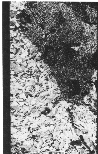
Fig. 2. Photomicrograph of section of cone structure illustrating orientation of feldspar lamination (field of view = 34 × 19 mm, partially crossed polars).
