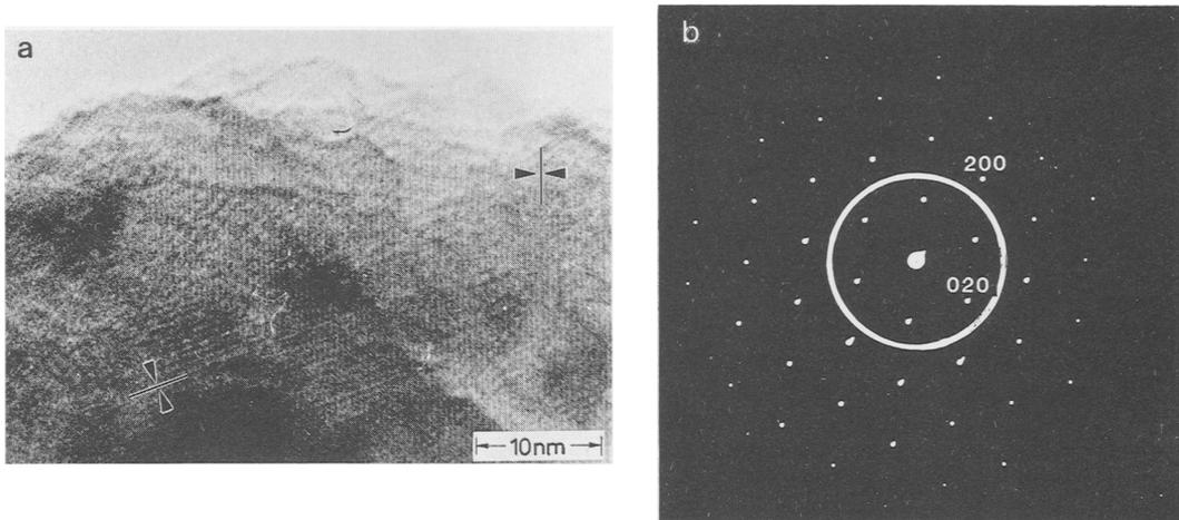
FIG. 2. (a) Lattice fringes from a portion of an aragonite crystal. (b) Corresponding electron diffraction pattern, [001] zone, of aragonite crystal shown in (a). The circle indicates the position of the objective aperture.
