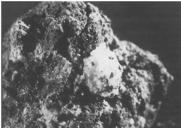
FIG. 1. Photograph of a typical encrustation (diameter approximately 5 mm) on a MSWI bottom ash sample. Ettringite, gypsum and gibbsite were identified in this sample.
