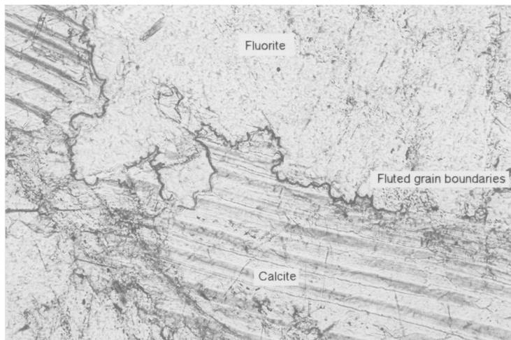
FIG. 1. Photomicrograph (PPL) of fluted grain boundaries (black line) between calcite, displaying truncated twin planes, and fluorite, representing replacement of the former by the latter. Field of view  $\approx 550 \times 800 \mu\text{m}$ .
