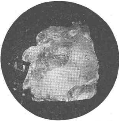
Fig. 1. Glassy quartz from Ducktown, Tennessee, showing strain structure.
