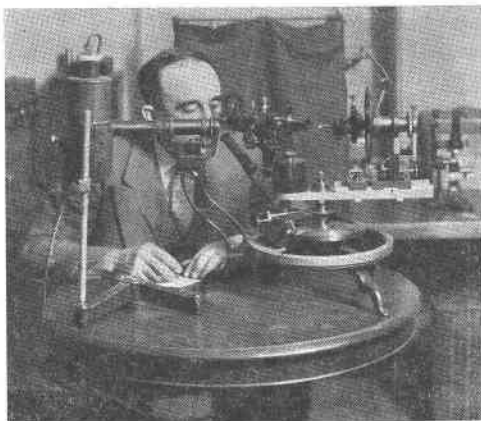
FIG. 1. Goniometer mounted on rotating table.
