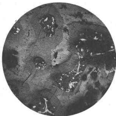
FIG. 3. Cores of stromeyerite (which has totally replaced tennantite) and native silver, surrounded first by galena and then by chalcopyrite. Vugs like the one represented by a black spot on the right ordinarily contain stromeyerite and silver. \times 60 (Photo by M. N. Short and R. W. Goranson).
