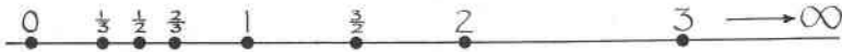
FIG. 1. Gnomonic projection of a normal zone having one principal node at infinity. Between the end-nodes 1, \infty , the derived nodes are spaced according to the terms of the normal complication series N_n .
