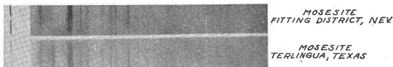
FIG. 1. Reproduction of diffraction patterns of mosesite from the Fitting District and from Terlingua.
