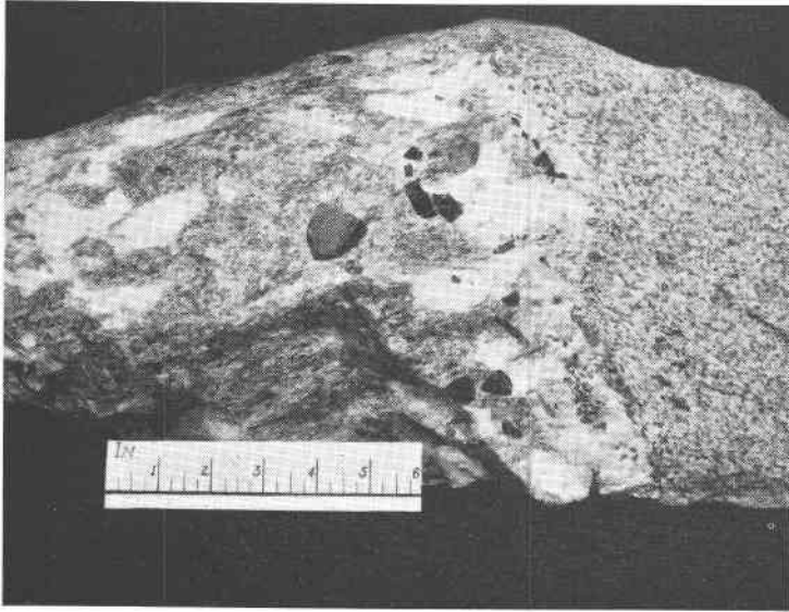
FIG. 3. Cross-section of a tourmaline type pegmatite showing white feldspar crystallized on the walls, and purplish-brown quartz occupying the center.
