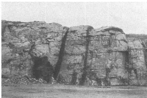
FIG. 1. A portion of the Lewiston City quarry showing trap dikes numbers 5 (left) and 6 (right). Height of quarry, 65 feet, distance between the dikes, 23 feet.
