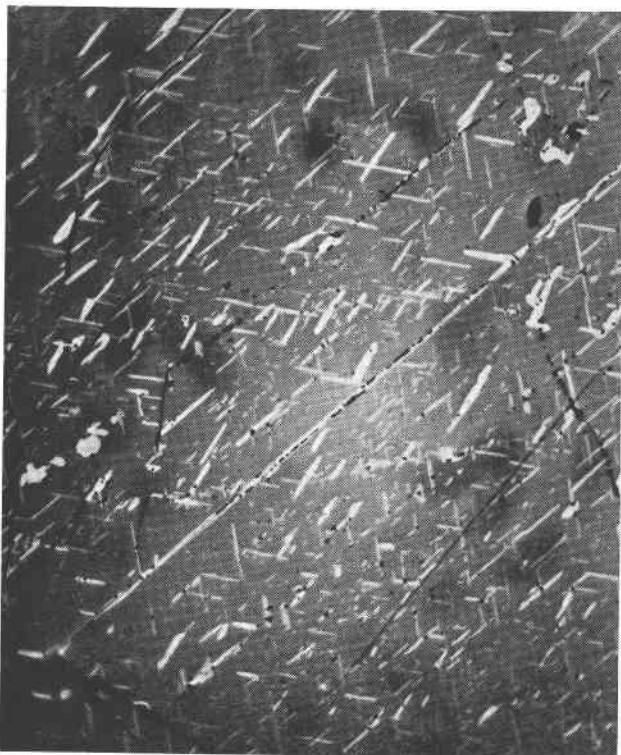
FIG. 2. Polished section of magnetite from the Nigger Hill Mine, U. S. Nat. Museum No. 11603, partially oxidized in air at 950^{\circ} – 1000^{\circ} . \times 740 . The bright portions are hematite, the ground is magnetite. The continuous narrow line of hematite running NE-SW marks an octahedral separation plane. The two parallel zones of more numerous short hematite lamellae, crossing the middle of the photograph nearly horizontally, mark the outcrops of two separation planes or potential separation planes parallel to the dodecahedron.
