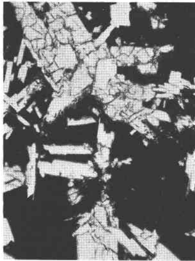
FIG. 9. Hill in Sec. 25, T 3 N., R 6 E. at elevation 3710 ft. Large pigeonite grains above and below; between plagioclase. The groundmass of glass is black from magnetite crystallites. \times 110 .
