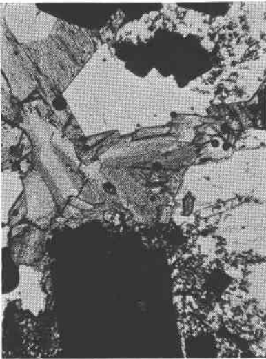
FIG. 3. Thin section showing black sitaparite, gray diaspore and white ephesite. \times 34 .
