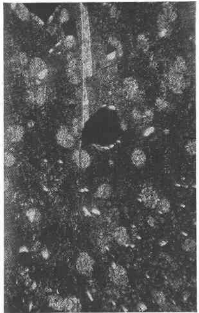
FIG. 4. Thin section of gamagarite with inclusions of hematite showing relict oolitic texture. \times 32 .
