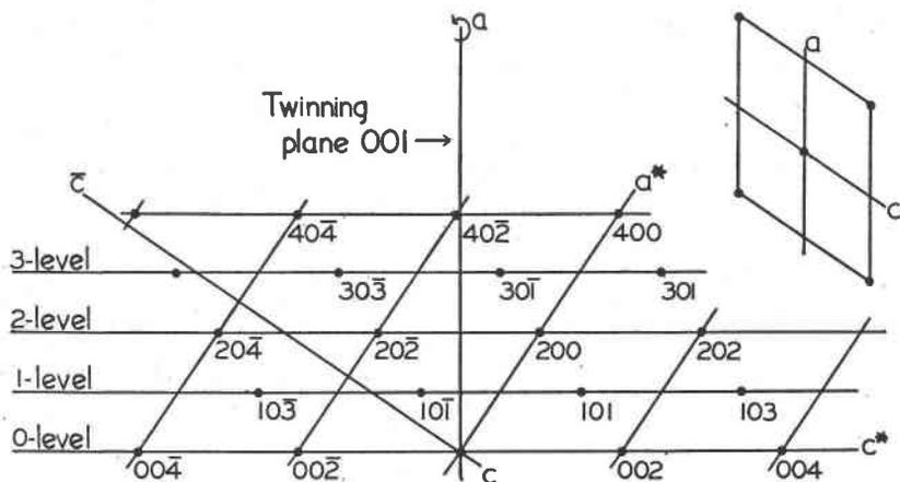
FIG. 2. Cross section through reciprocal lattice, showing sequence of levels in the  $a^*-c^*$  plane. Rotation axis is  $a$ .
