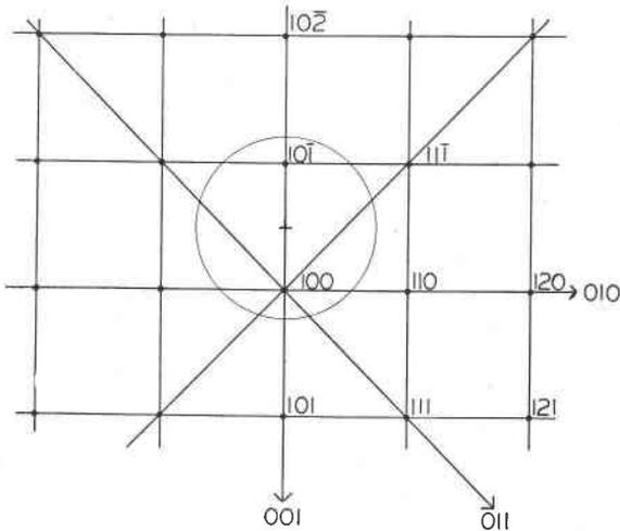
FIG. 7. Gnomonic projection perpendicular to the  $a$  axis. The points do not represent observed faces, but merely internal planes. Poles  $100$  and  $10\bar{1}$  are nearly equidistant from the projection center, resulting in a pronounced pseudo-symmetry. Because of the near equivalence of  $b$  ( $6.92\text{\AA}$ ) and  $c \sin \beta$  ( $6.86\text{\AA}$ ) the projection appears tetragonal.
