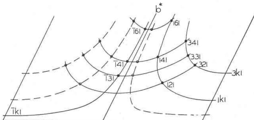
FIG. 5. Diagrammatic representation of 1-level Weissenberg photograph about the  $c$  axis of type 2 crystal. Solid points represent reflections from one twin (100) orientation; circles represent reflections from the other orientation.
