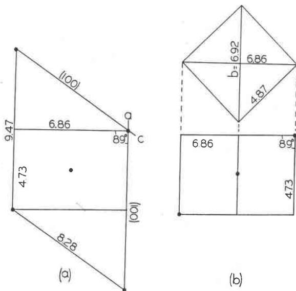
FIG. 6. (a) Cross section through *B* cell, showing relation to pseudo-orthorhombic unit. (b) Diagram showing relation of pseudo-orthorhombic unit to the pseudo-cubic unit.
