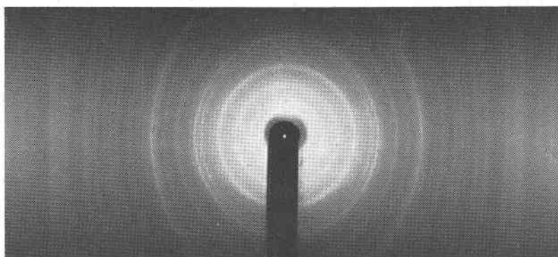
FIG. 3. C. Orängeite, Arö, near Langesund, Norway. Heated 40 hours at 650° C. "Single crystal" rotation pattern. Tetragonal \text{ThSiO}_4 only. E. Orangeite, Madagascar. Unheated. "Single crystal" rotation pattern. Tetragonal \text{ThSiO}_4 only.
