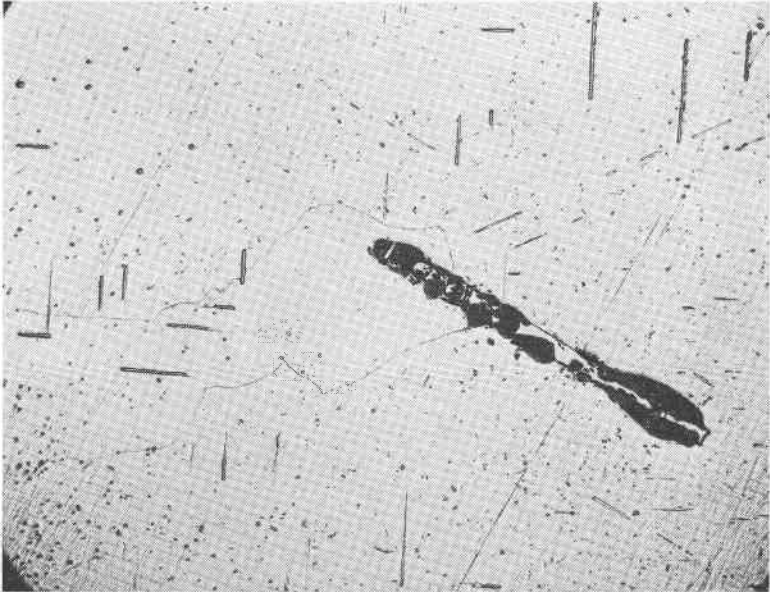
FIG. 7. The big inclusion is rhabdite, perhaps large enough to be called schreibersite, the dark spots are due to chipping in the preparation of the surface. If the plane of the picture is parallel to 001, the small rhabdites at right angles to each other lie along the cube face and the large phosphide body and the other rhabdites are parallel to trapezohedral faces. \times 40 .
