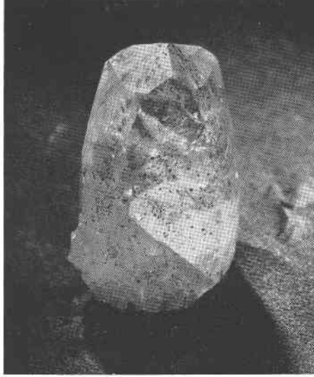
FIG. 1. Smythite inclusions in calcite crystal from the Bloomington Crushed Stone quarry. The sharper scalenohedral habit of the earlier calcite (I) can be seen outlined in phantom by the smythite near the top of the crystal.
