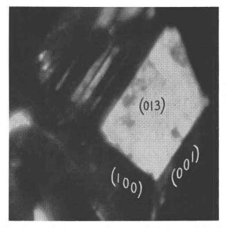
FIG. 1. Photomicrograph of a typical  $\beta$ -Ga<sub>2</sub>O<sub>3</sub> crystal. The faces are indexed after the monoclinic unit cell. The zone of reentrant angles lies in  $\{0kl\}$ . (570×).
