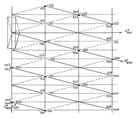
FIG. 2. Portion of the  $\beta$ -Ga<sub>2</sub>O<sub>3</sub> reciprocal lattice showing the relationship between monoclinic and orthorhombic symmetry. Upper monoclinic cell (dashed) lattice points (open symbols) are indexed to the upper left of each permissible lattice site; lower monoclinic cell (solid, heavy) lattice points (solid symbols) are indexed to the lower left; orthorhombic unit cell (solid, light) lattice points are indexed to the right.
