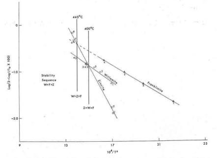
FIG. 2. Plot of the reciprocal absolute temperature against the log of the absorbance for franklinite, willemite, and zincite from Sterling Hill, New Jersey.
