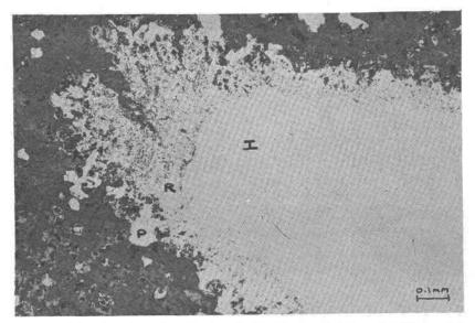
Fig. 1. Broad reaction rim developed about magnesian ilmenite (I), consisting of an outer zone of pure perovskite (P) and an inner zone of perovskite, ilmenite and ferromagnesian silicates (R). Bultfontein pipe, South Africa.
