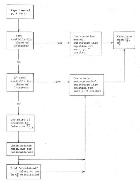
FIG. 1. Scheme of calculation of thermodynamic parameters for minerals from hydrothermal equilibrium data.
