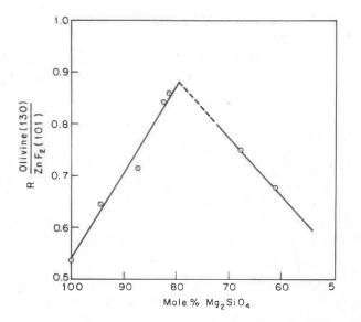
FIG. 1. Mole percent  $M_{\mathfrak{Z}_2}SiO_4$  vs.  $R = \frac{\text{integrated intensity olivine (130)}}{\text{integrated intensity } ZnF_2 (101)}$
