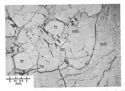
FIG. 1. Photomicrograph showing a large, heavily fractured area of mooihoekite (dark grey, mh) separated by a curving fracture from an area containing an intergrowth of mooihoekite (dark grey, mh) and haycockite (light grey, hc). The rounded light grey areas extending from the top left corner are troilite (tr).
