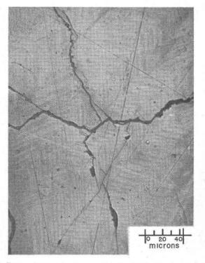
FIG. 3. Photomicrograph showing details of twinning in haycockite.
