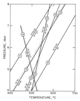
Fig. 3. Pressure-temperature diagram for reactions in the CaO-Al<sub>2</sub>O<sub>3</sub>-SiO<sub>2</sub>-H<sub>2</sub>O system. Reactions have been modified for solid solution. Stable assemblages of phases in reactions indicated by stippling on stable side of reaction curve. For example, zo + ky is stable in reaction (12).
