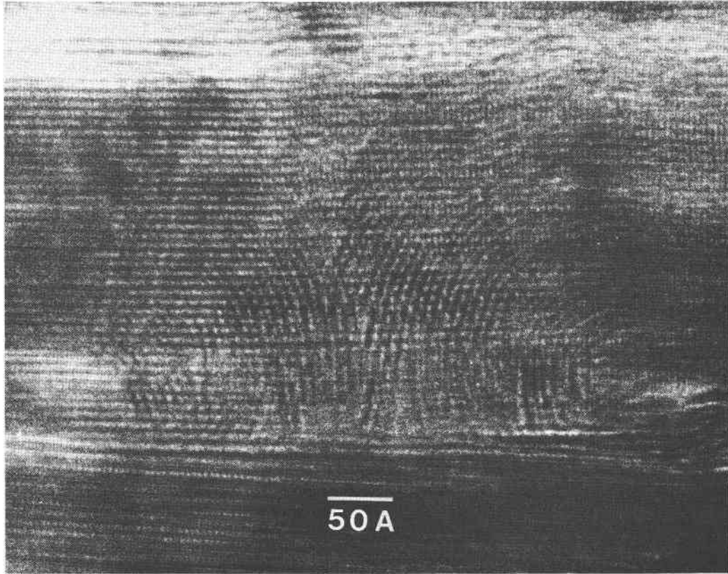
Fig. 25. Romanian uralite. Crossing of (001) fringes from planar and curved serpentine. Features such as this suggest that the serpentine is a ribbon structure, as shown in Figure 26.
