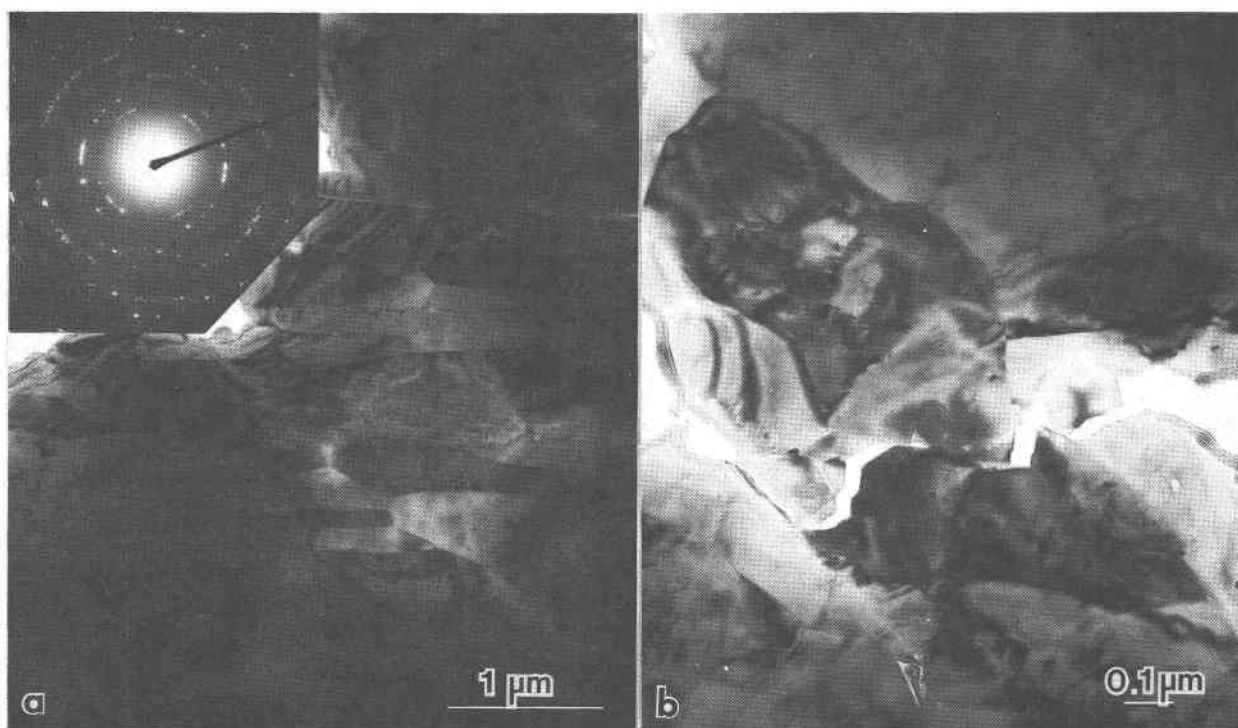
Fig. 3. Cortex of ooids consisting of fine grained calcite in Twin Creek oolite. (a) Radial fabric of calcite needles with considerable preferred orientation as shown by the SAD; (b) Micritic calcite fabric of cortical coatings.
