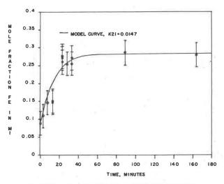
Fig. 3. Disordering with time at 700°C, Sample TZ.
