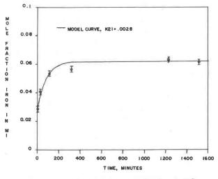
Fig. 4. Disordering with time at 700°C, Sample HC.
