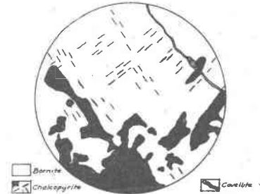
Fig. 4—Showing the development of finger-like masses of chalcopyrite with rectilinear extensions parallel to the orientation of the chalcopyrite needles.
