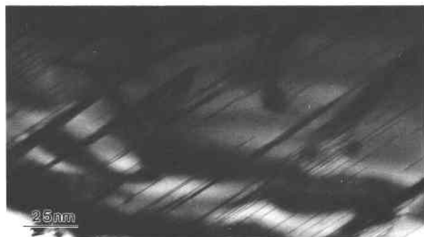
Fig. 4. An area of an olivine crystal containing abundant dislocations that are decorated by layers parallel to (001) olivine.
