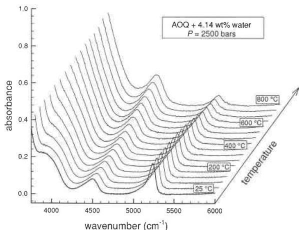
**FIGURE 3.** Near-infrared spectra of a haplogranitic sample (labeled AOQ) with normalized anhydrous composition of 4.65 wt% Na<sub>2</sub>O, 5.68 wt% K<sub>2</sub>O, 13.53 wt% Al<sub>2</sub>O<sub>3</sub>, and 76.14 wt% SiO<sub>2</sub>, containing 4.14 wt% H<sub>2</sub>O<sub>tot</sub> from 800 to 25 °C at 2500 bars collected during the cooling period.
