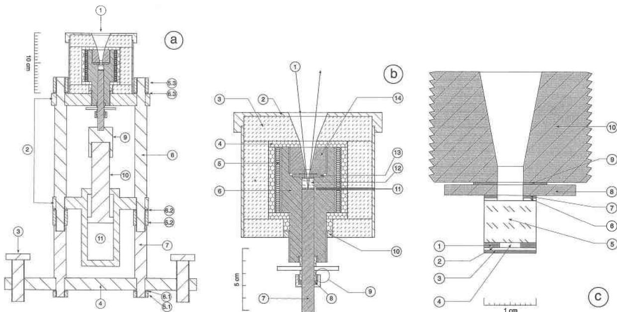
**FIGURE 1.** (a) Schematic drawing of the new cell assembly: 1 = the cell, 2 = flanges, 3 = adjustable screw, 4 = base plate, 5.1–5.3 = nuts, 6.1–6.3 = washers, 7 and 8 = steel poles, 9 = coupling, 10 = oil hydraulic piston, and 11 = oil hydraulic cylinder. (b) Details of the cell: 1 = near-infrared beam, 2 = aluminum pot, 3 = isolation made of mullite wool, 4 = pyrophyllite box, 5 = heating coil, 6 = cell cylinder, 7 = hard metal
