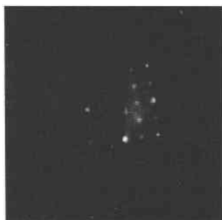
FIGURE 2. LEED pattern obtained from a clean FeS 2 (100) surface at an electron-beam energy of 125 eV. The middle [(0,0) beam] and left portions of the pattern are obscured by the sample holder.
