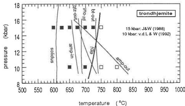
**FIGURE 6.** Pressure-temperature diagram for trondhjemite at H<sub>2</sub>O-saturated conditions,  $f_{O_2}$  unbuffered. Compiled from Johnston and Wyllie (1988) and van der Laan and Wyllie (1992).
