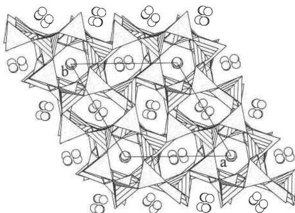
FIGURE 3. Crystal structure of trinepheline as viewed down *c*. Open circles indicate the Na ions.
