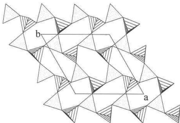
FIGURE 2. Single tetrahedral layer of the trinepheline structure ( $0.19 \leq z \leq 0.41$ ). Hatched and stippled tetrahedra correspond to SiO<sub>4</sub> and AlO<sub>4</sub> groups, respectively.
