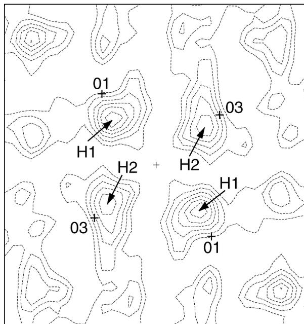
**FIGURE 4.** Difference Fourier map calculated for neutron powder diffraction data using only the akaganéite octahedral framework as the model structure, at  $y = 0$ . For clarity, only the negative contours are plotted. The contour interval is 0.1 scattering units.
