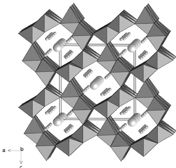
**FIGURE 1.** Polyhedral representation of the akaganéite structure, looking approximately down **b**. The small circles represent the H atoms, and the larger circles in the tunnel region indicate Cl anions.
