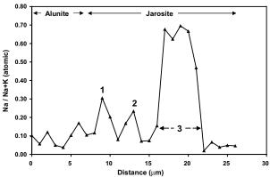
**FIGURE 3.** False-color BSE image magnifying the central area of Figure 2, and corresponding plot of EDS EMP traverse with a 1  $\mu$ m beam. The plot shows the traverse with respect to Na/Na + K (atomic) and highlights the locations of points 1, 2, and band 3 on the image.
