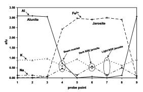
**FIGURE 1.** BSE image of alunite (A) and jarosite (J) and corresponding WDS EMP analyses with a 10  $\mu$ m beam. The plot shows jarosite and alunite compositions with respect to Fe<sup>3+</sup>, Al, K, and Na reported in atoms per formula unit (afu). Representative complete analyses from this figure are reported in Table 1 where, for example, probe point 1-9 refers to Figure 1, point 9. Note the overgrowth of jarosite (light) over alunite (dark) in the lower central part of the BSE image.
