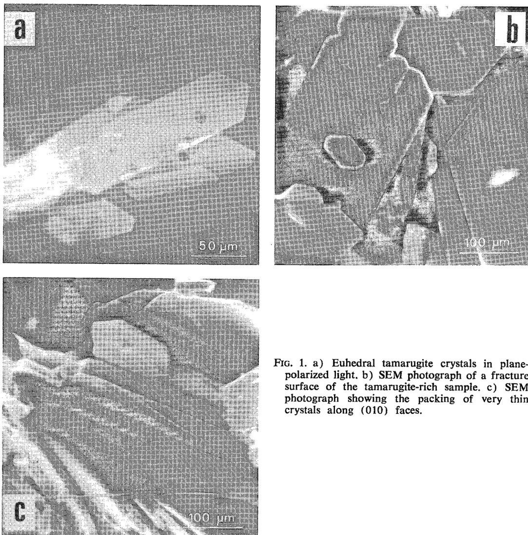
Fig. 1. a) Euhedral tamarugite crystals in plane-polarized light. b) SEM photograph of a fracture surface of the tamarugite-rich sample. c) SEM photograph showing the packing of very thin crystals along (010) faces.
