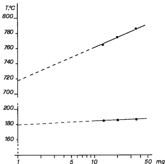
FIG. 3. Dependence of peak temperature on sample weight for the main thermal effects of tamarugite.
